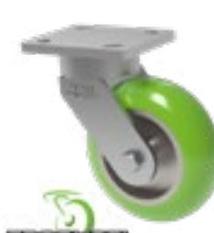
ErgoXcel™ is our line of maintenance-free casters that never need greasing or any type of service. They feature precision neoprene sealed ball bearings and hardened raceways, ensuring smooth rotation for several years. The rounded tread that ErgoXcel™ features increases ergonomic benefits by reducing force exerted to keep rolling, as well as dispelling debris.
