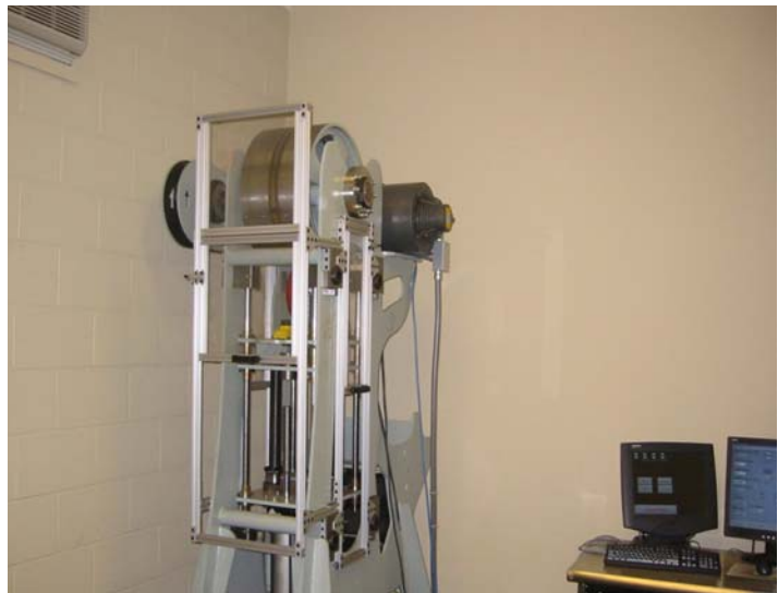
Figure 1: Wheel Endurance Test Machine at CCI
