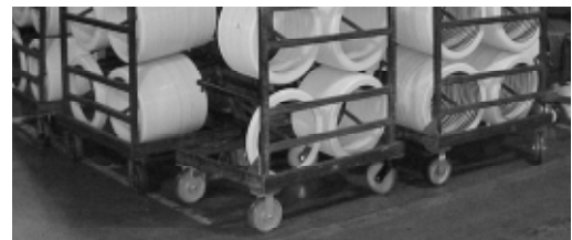
Cantilever racks holding parts for production with 51 Series casters.
