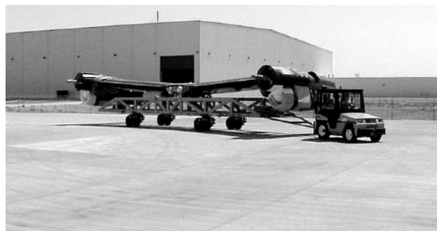
Dual pneumatic casters supporting an aircraft wing dolly.
